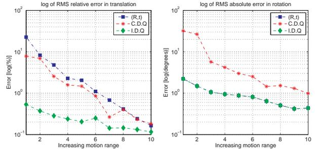
Fig. 4. Effect of the motion amplitude in the estimation error of the hand-eye transformation. The motion amplitude increases in successive trials. The standard deviation of the translation component goes from 10 mm to 100 mm in steps of 10mm, while the angle of the rotation increases from  $10^\circ$  to  $55^\circ$  in steps of  $5^\circ$ .
