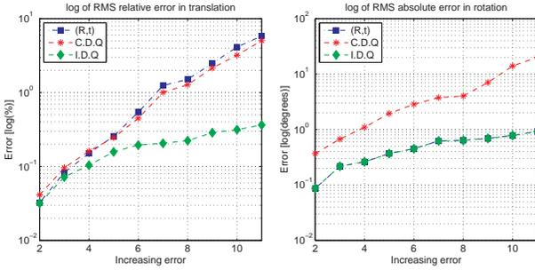
Fig. 2. Accuracy of the hand-eye computation in the presence of noise in the motion estimation. The standard deviation of the additive noise in translation increases from 0 mm to 9 mm in steps of 1 mm, while the noise in rotation increases simultaneously from  $0^\circ$  to  $2.25^\circ$  in steps of  $0.25^\circ$ .
