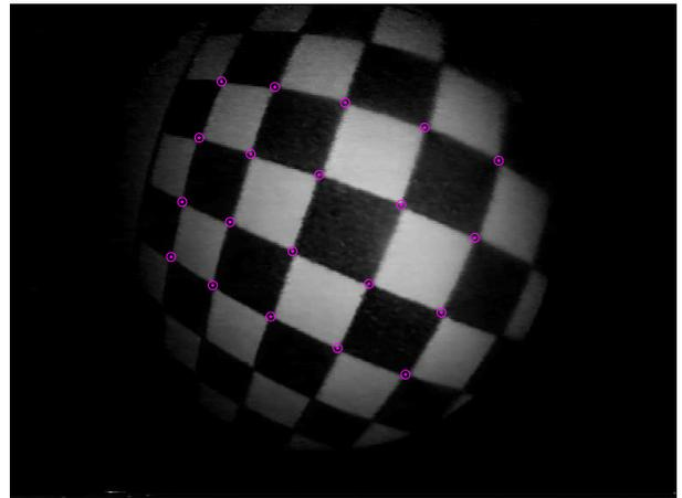
**Fig. 1.** Endoscopic image exhibiting strong non-linear lens distortions. User selects grid points (red) for calibration.
