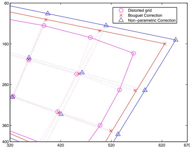
**Fig. 4.** Undistortion performed to user selected points in the acquired image using Bouguet calibration (using radial distortions) as well as the non-parametric approach. Bouguet underestimates the distortions and consequently the points do not lie on a straight line. In contrast the non-parametric approach performs better.
