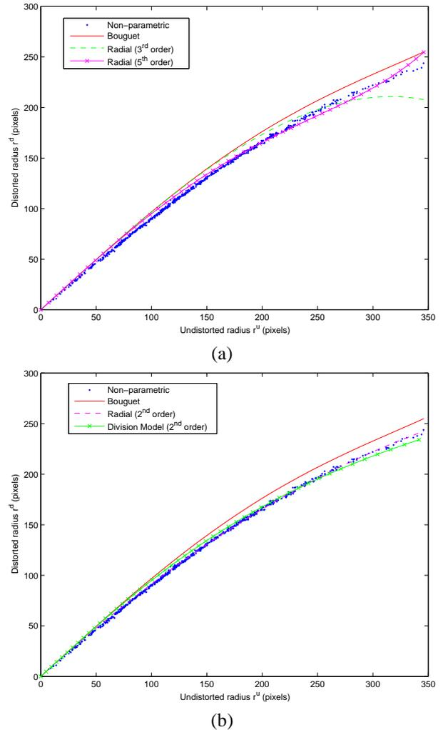
**Fig. 3.** Fitting of various distortion models to the estimated distortion curve. In (a) we fit the standard 3<sup>rd</sup> order, and 5<sup>th</sup> order radial distortion models to the distortion profile. In (b) we compare between the radial model used in the Bouguet toolbox, the division model and a simple quadratic model. From these plots it is clear that conventional models do not fit the radial distortion profile well.
