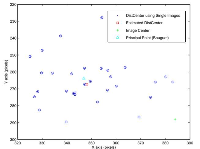
**Fig. 2.** Plot showing the variance in the estimated center of distortion across the set of acquired images. The centers are individually estimated by decomposing the individual fundamental matrices as described in Section2. Also shown are the effective distortion center computed using all the  $F$  matrices simultaneously and the principal point estimated using Bouguet[9].
