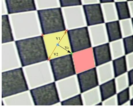
Figure 5: Direction definition. The direction is defined by finding the yellow corner point on the left side of the vector joining the centroid to the origin corner.
