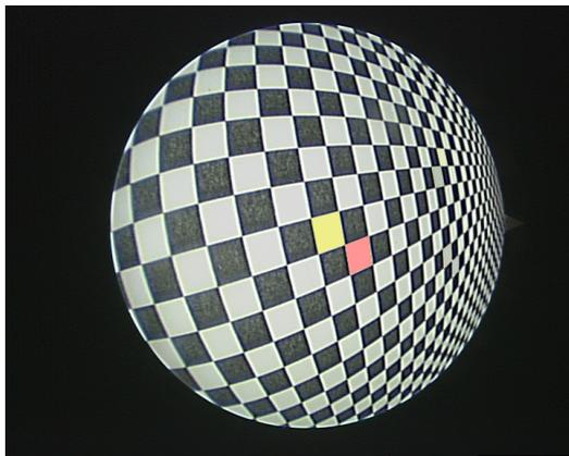
Figure 1: Synthetic image used to test the algorithm. The grid has two painted squares (one yellow and other pink) used in the origin and direction detection.
